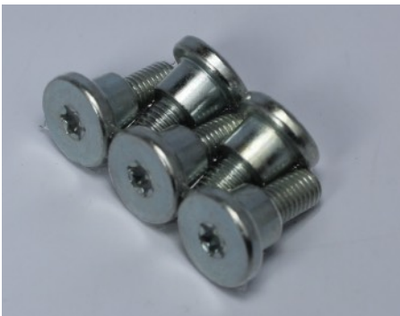
Part No. 3572-5 FRONT BRAKE ROTOR MOUNTING KIT Custom button head style zinc plated torx screws replace OEM 3762M used on 2006-up Dyna with cast wheel only.
