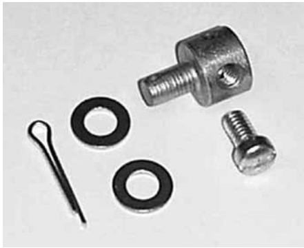
Carburetor Throttle Lever Wire Block Cadmium plated duplicate of OEM 27450-36 block, screw, cotter pin and brass washers used on all Linkert and Bendix carburetors. Stock No. 2658-5 Standard Size Stock No. 2664-5 Oversized \pm .005
