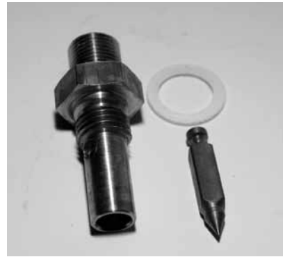
Carburetor Float Valve and Seat Reproduction of OEM 27382-33 float valve and seat, OEM 27402-33 gasket used on 1933-1965 Linkert carburetors. Stock No. 2880-3
