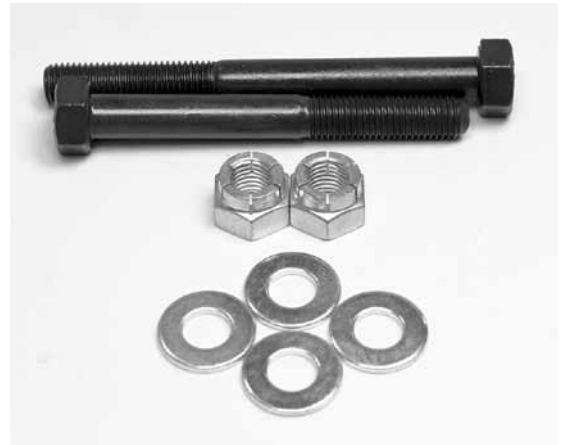
Gas Tank Mounting Kit Parkerized 1038 bolts 4072 and 4082, cadmium 6320 washers, 7725 flexloc nuts used on 1952-1978 K, KH, Sportster. Correct OEM spacers available as needed. Stock No. 3474-8
